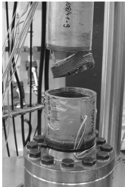
Figure 4. Failed connection after fatigue test
