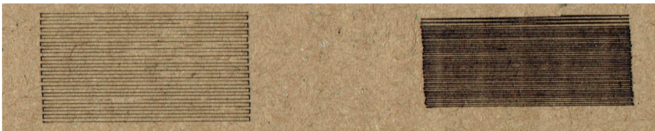
Figure 11. Different line density in filled laser marking on cardboard (3 lines/mm left, 6 lines/mm right)
