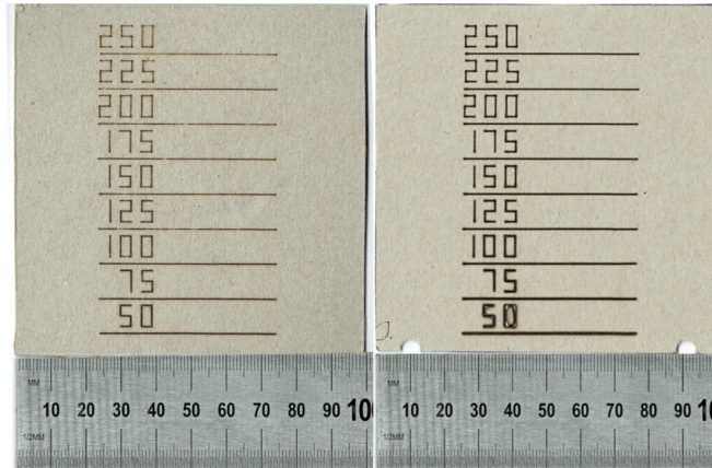
Figure 8. Speed test on cardboard (0.5W left, 2.5W right), numbers mm/min feedrate
