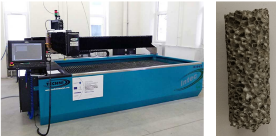
Figure 3. The TECHN I510-G2 abrasive water jet cutting machine and the specimen (AFBFs)
