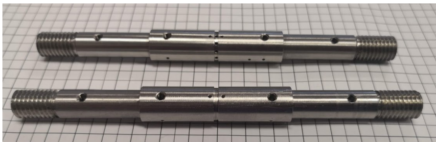
Figure 2. Simplified geometry for the electrical resistance without and with holes
