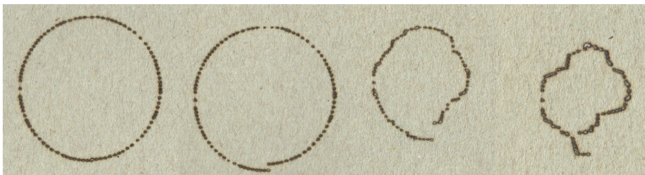
Figure 7. Negative effect of increasing the feedrate: 400, 420, 450, 500 mm/min
