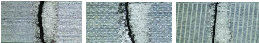
Figure 6. Fretted area after failure ( F_N=543\text{N} , F_{fat}=8.8\text{kN} ). Left: virgin; middle: point pattern; right: line pattern
