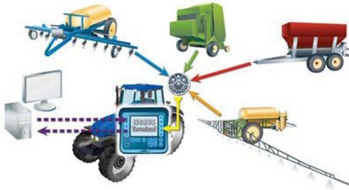
Figure 1. Connection possibilities based on ISO 11783 (Source: TeeJet, 2010.)
