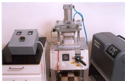
Figure 1. Pneumatic opening and closing press equipment tool with tool heating by heating flat
