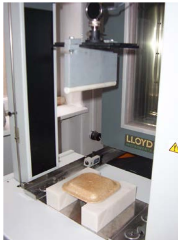
Figure 6. LLOYD LR5K PLUS computer-controlled universal tensile machine prepared for breaking test (Central Environmental And Food Science Research Institute, Budapest)
