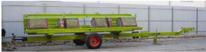
Figure 1. Trailer adapted for acceleration measurements
