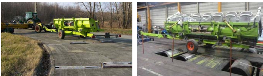
Figure 5. Measurements on circular track and rolling testbench
