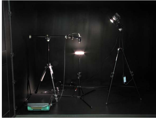
Figure 3. Light-isolated measurement cabinet
