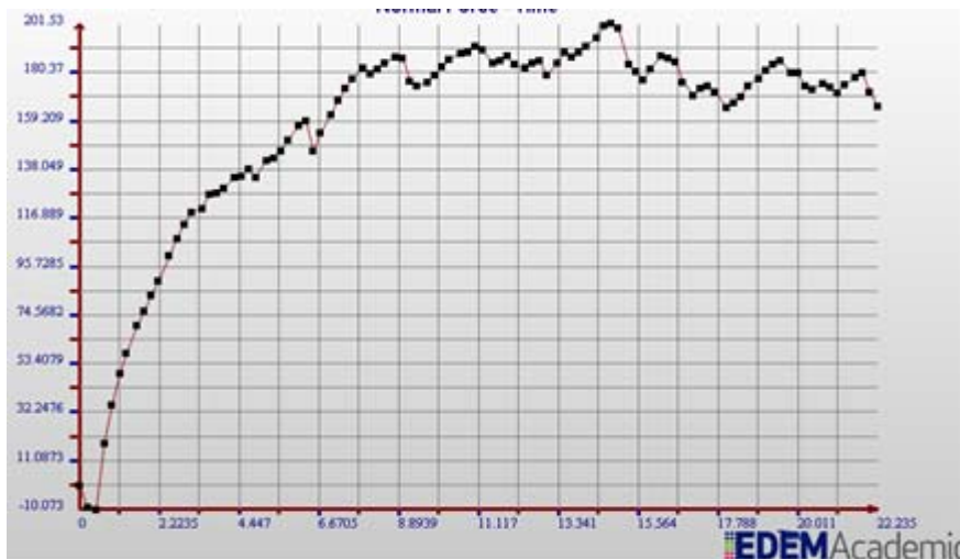
Figure 6. Shear force – time diagram from the DEM model, critically consolidated sample
