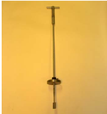
Figure 4. Soil shearing test instrument with the mass
