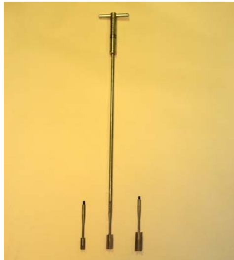
Figure 3. Torsional soil shearing instrument with three rungs
