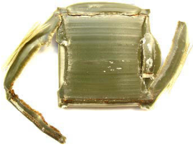
Figure 13. Overloaded ( p=150 MPa, v=5 mm/s) PA specimen against steel
