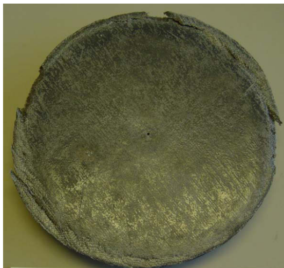
Figure 12. Failure mechanisms of highly loaded fibre reinforced polyester
