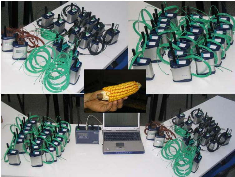
Figure 3. Assembly of the measuring ports for measuring the temperature and humidity of drying air and the temperature of material
