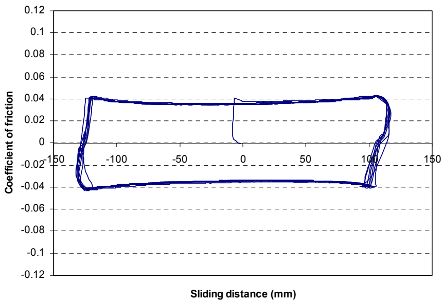
Figure 9. Friction curve of UHMWPE against Steel St 37.2
