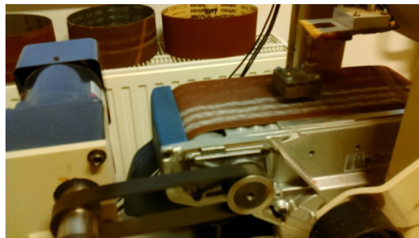
Figure 1. Pin-on-plate wear device.
