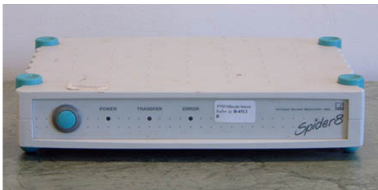
Figure 3. Spider 8, a strain gage measurement device
