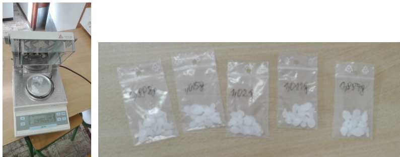
Figure 1. Sartorius MA30 digital scale and paraffin masses used for measurements
